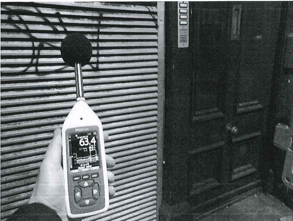
Figure 4: Plant noise at 1m.
